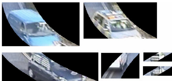
Figure 6: Reconstructed image patches of tracked vehicles. The size of the patches can be customized to display as much of the vehicles as desired.
